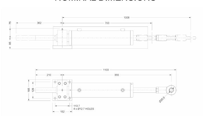
NOTE: dimensions are nominal only and subject to change without notice. These dimensions should be used only as a general guide to the footprint of space required. Final drilling and fitting of the cylinder should only done once the unit has been delivered and on-site.
