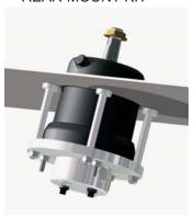
REAR-MOUNT Kit - fits any model 501 & 502 helm unit - adjustable from lowprofile to full protrusion for maximum flexibility in helm placement. Simply trim the spacers and studs to adjust the amount of penetration into the helm position. The front dash or console ring is fully O-ring sealed against pump body to prevent water ingress to the rear of the console. Easy to fit - easy to adjust - looks great.
