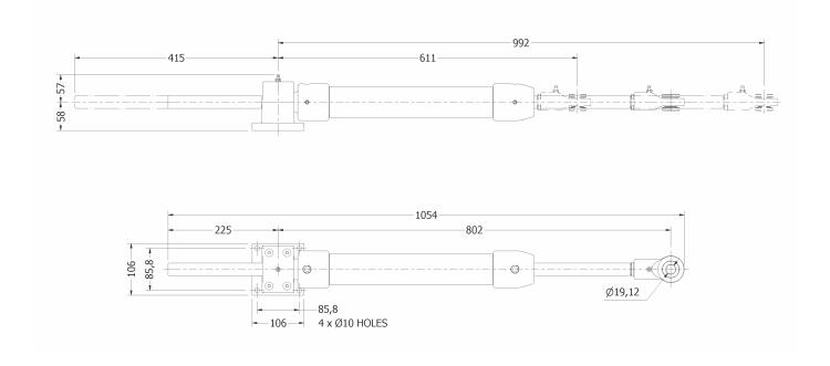
NOTE: dimensions are nominal only and subject to change without notice. These dimensions should be used only as a general guide to the footprint of space required. Final drilling and fitting of the cylinder should only done once the unit has been delivered and on-site.
