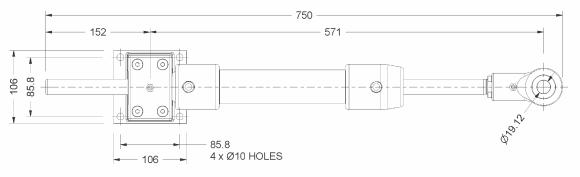
NOTE: dimensions are nominal only and subject to change without notice. These dimensions should be used only as a general guide to the footprint of space required. Final drilling and fitting of the cylinder should only done once the unit has been delivered and on-site.
