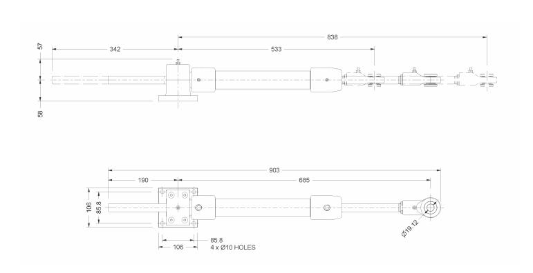
NOTE: dimensions are nominal only and subject to change without notice. These dimensions should be used only as a general guide to the footprint of space required. Final drilling and fitting of the cylinder should only done once the unit has been delivered and on-site.
